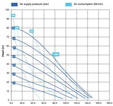
\* The curves and performances refer to pumps with submerged suction and free delivery outlet, with
