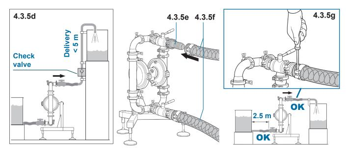
4.3.5g Connect the food-grade certified hoses to the rigid system pipes (suction and discharge) upstream and downstream of the pump. Check that the system ducts are fixed and self-supporting and that they do not weigh on the pump.
