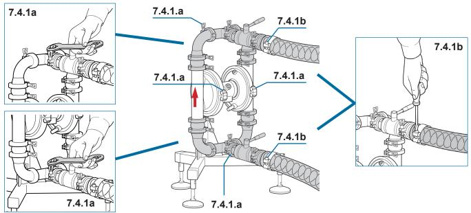
7.4.1a Using a suitable spanner, check the tightness of the pump body clamps and the pump suction and delivery manifold clamps.
