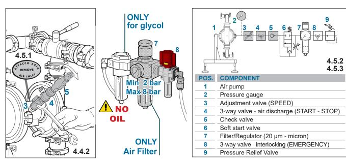
Tighten a compressed air flow control valve, a 3-way valve (START - STOP with air discharge) and a check 4.5.2 valve on the pneumatic circuit connection of the pump, as per the diagram in the figure. Install a pressure gauge on the compressed air connection of the pump itself and check the value with the pump running to check the actual pressure of the supply air.
