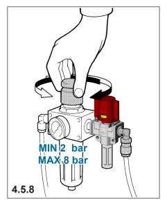
4.5.8 Adjust the network pressure of the compressed air to guarantee pressures of not less than 2 bars and not more than 8 bars when the pump is running.
