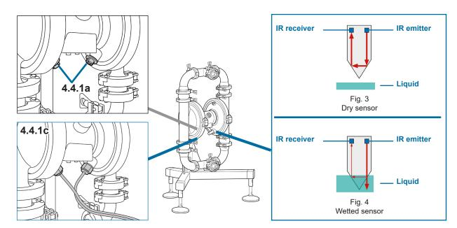
To install the optical "Diaphragm rupture" detection sensors on the pump, proceed as follows:
