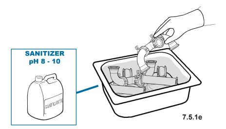
The internal manual pump washing is now complete; reassembly is possible.
