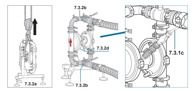
7.3.2d If the pump is equipped with diaphragm rupture sensors, the connection of the electrical signal connectors must be reset.
