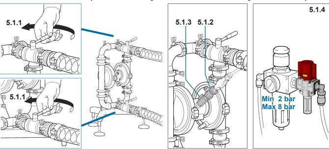
5.1.1 Open the product shut-off valves of the suction and delivery pipes.
