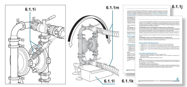
6.1.1m Reconnect the suction and delivery lines of the processing system to the respective pump connections and secure them with the appropriate clamps.
