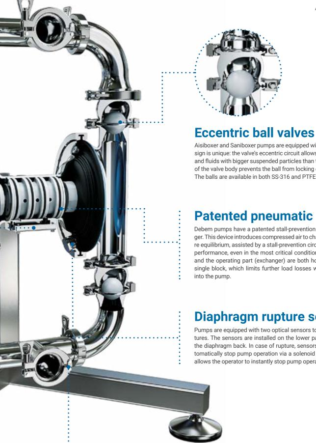
Aisiboxer and Saniboxer pumps are equipped with ball fluid valves. Their design is unique: the valve's eccentric circuit allows to handle higher flow rates and fluids with bigger suspended particles than the normal. The eccentricity of the valve body prevents the ball from locking during pumping operations. The balls are available in both SS-316 and PTFE.
