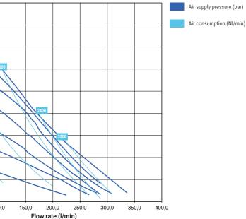
\*The curves and performances refer to pumps with submerged suction and free delivery outlet, with water at 20° and vary according to the
