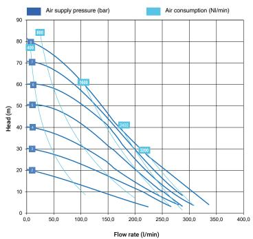
\*The curves and performances refer to pumps with submerged suction and free delivery outlet, with water at 20°C and vary according to the composition materials.
